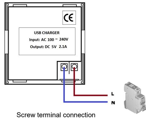
**Note:** It is recommended to install this socket as terminal equipment in the circuit.
